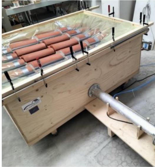
Wooden plenum chamber (internal dimensions 170x120x60 cm) connected to an iron pipe 3,5m long ( \varnothing=90\text{mm} )
